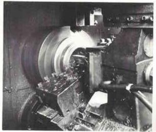
Once we're satisfied that the experimental machines meet all of the predetermined requirements, we begin tooling up for production. Nearly all tooling is done in our ultra-modern factory in Fargo. Tools are built to exacting, precision specifications. For instance, once we know that precision parts meet exacting tolerances, we computer program this automatic turret lathe to machine components to the desired tolerances.
