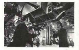
It must be a hefty bolt to require a five-foot-long torque wrench. It is. It's the bolt that holds the Steiger drawbar to the tractor. Nearly twice as large as drawbars used in some competitive tractors.
