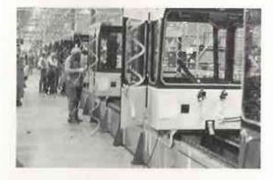
Steiger Safari cabs must be properly constructed. They become the business office of the end user — the farmer. They're built with the same simple, exacting practices that are found in the rest of the tractor. Notice the bulk of the rails on which they are assembled. Gives you just a clue as to the strength of the cab.
