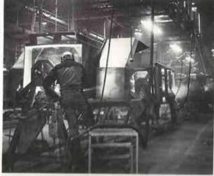
Weld jigs allow frames to be lurned, so welders never have to work overhead. Everything is done in the most convenient, efficient manner, which lets Steiger produce a superior product. These jigs also perfectly position sub-assemblies, so interfacing during later assembly is easily accomplished.
