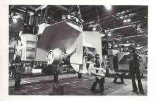
When a Steiger tractor reaches the end of the line, it still can't go anywhere on its own, because it has no wheels. So, we gently pick it up and move it to a hydraulic lift, a lot like the one in your neighborhood service station, but a lot bigger. Here, we put on the wheels, snug up bolts and assemblies in the undercarriage, and get the tractor ready to drive out the door. Easy as pie!
