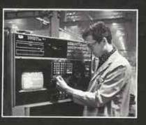
Raw castings, such as axle housings and power divider castings, are automatically machined, drilled and tapped by computer-controlled equipment. This machine, programmed and operated by computer tape, automatically selects the right cutter, drills and taps to the proper depth, and turns lhe castings to the proper angles for precision milling. It is typical of the Steiger manufacturing process - just one of the advanced techniques employed to produce quality products at an equitable price.
