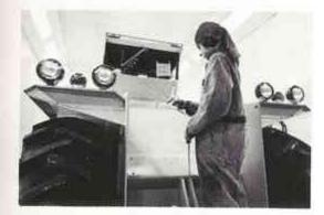
During final assembly stages, paint is going to become a little soiled, maybe scratched in a place or two. Quality control won't let it go out the door in that condition. All exposed surfaces are carefully inspected, and all blemishes painstakingly corrected. Then it undergoes another inspection, to make sure nothing is accidentally missed.
