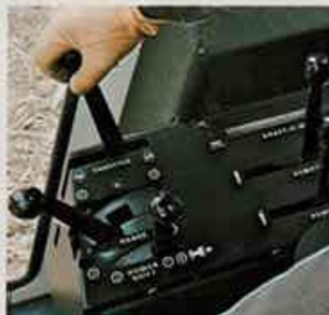
Control panel (right-hand) includes remote for power shift, range shift, mode, Differential Lock, Differential Locking, two remote hydraulic circuits, power take-off.
