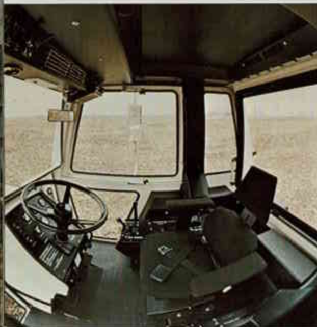
Pedal-operated tilt/telescoping wheel slips out of the way for easy access, adjusts to suit your height, size and leg length. Tilt from 05° to 90°, telescopes in or out five inches to five different positions.
