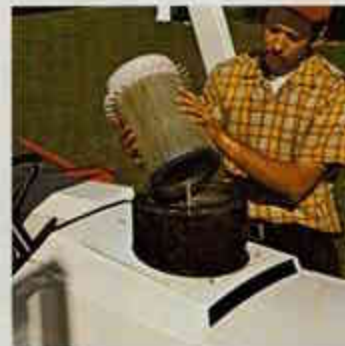
Giant 67-type air cleaner has safety-type double element. It's 98.9% efficient. Serviced in a jiffy—gauge tells you when—no messy oil. Vacuum valve automatically unloads dust from body. Mounted below eye level. Pre-cleaner is optional.
