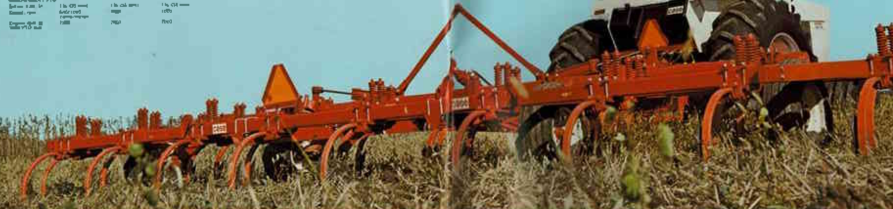
Up to 168 inch spread traps. With the optional 20 inch axle and 12 1/8 inch wheel spacing, you can move 48-inch traps out to a full 152 inches center-to-center frame. They're used in slip-rice paddy cultivation and can be used in many other specialized wide-row applications.
