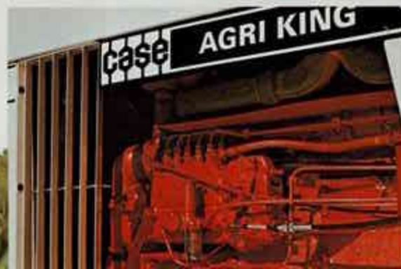
New heat shield (1270/1370) between fuel system and exhaust manifold holds down fuel temperatures to boost engine performance.
