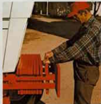
Implement side mounting rails and sliding weight attachments. Heavy-duty 250 pound side rails provide solid foundation for chemical tank supports. Front weight frame weighs 374 pounds, slides in and out to add, move or remove 75 pound weights of hang-in design. Side rails standard on 1270 and 1320, sliding weight attachment optional; all are optional on the 1175.
