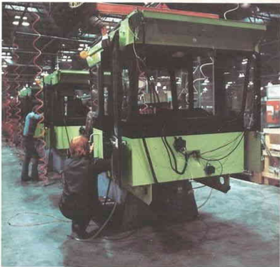
Assembly of tractor cabs at Steiger's Fargo plant
